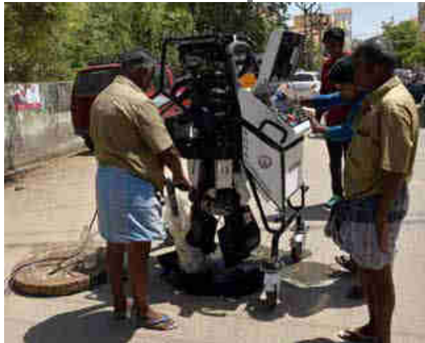
COIMBATORE: To stop manual scavenging, the Coimbatore Municipal Corporation is now using Robots to clean blocked drains in the city. Sanitary workers are provided with a bot, controller and a screen to clean the manholes without coming in contact with the toxic gasses. The bot has the capacity to go as deep as 20 feet to clean clogged drains.
